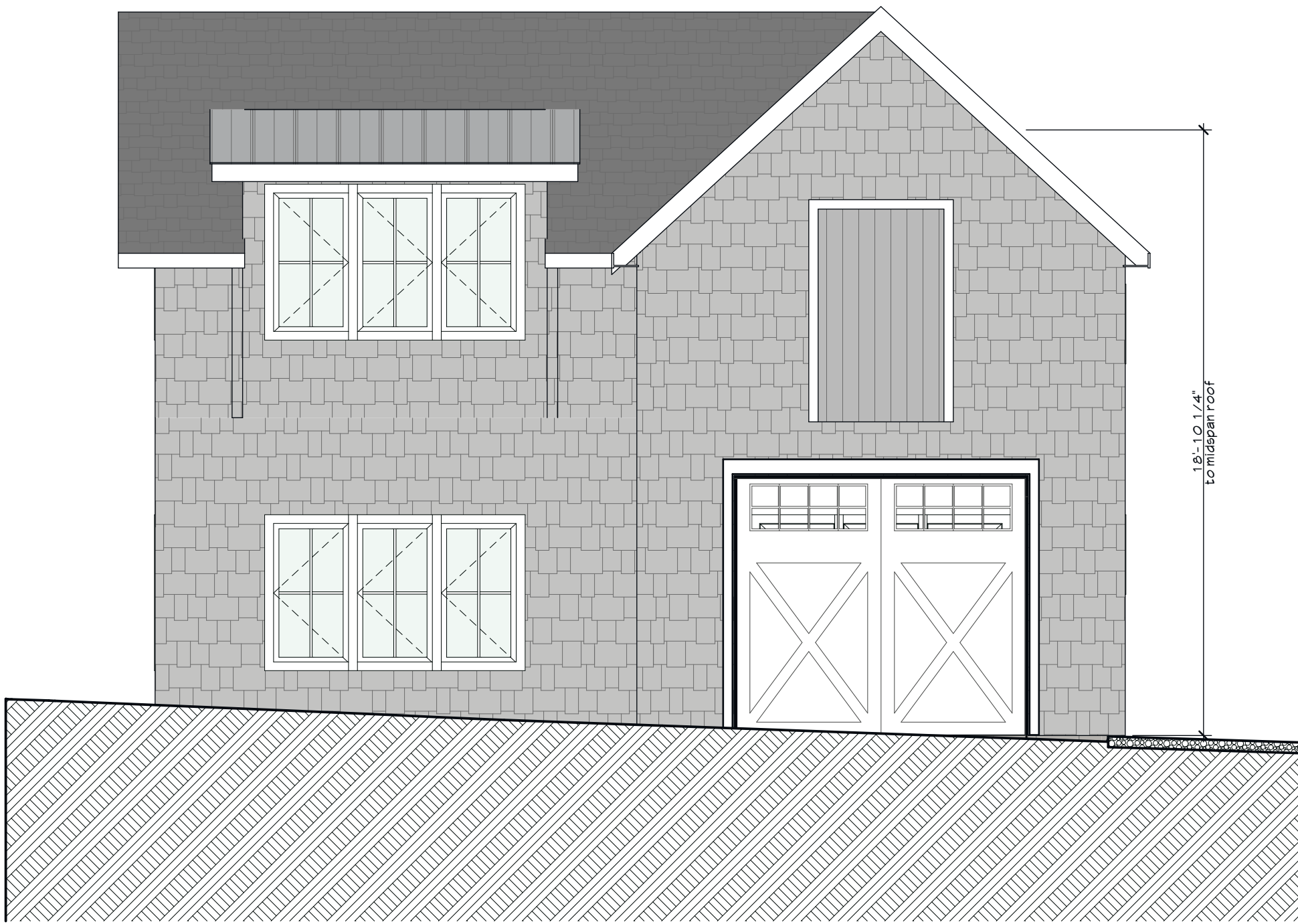
SEA 2.04 South Elevation-Garage SCALE: 1/4" = 1'-0" 0 2' 4' 8'
