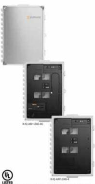
The Enghane IQ Combiner 4/4C with Enphase IQ Gateway and integrated LTE-M1 cell modern (included only with IQ Combiner 4C) consolidates interconnection equipment into a single enclosure and streamlines IQ microinverters and storage installations by providing a consistent, pre-wired solution for residential applications. It offers up to four 2-pole input circuits and Enton BR series busbar assembly.
