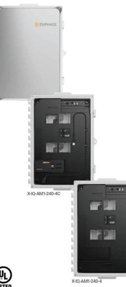
The Enphase IQ Combiner 4/4C with Enphase IQ Gateway and integrated LTE-M1 cell modem (included only with IQ Combiner 4C) consolidates interconnection equipment into a single enclosure and streamlines IQ microinverters and storage installations by providing a consistent, pre-wired solution for residential applications. It offers up to four 2-pole input circuits and Eaton BR series busbar assembly.
