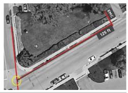
lines, as extended. The distance shall be measured along the right-of-way line from the point of intersection. (See graphic illustration above.)
